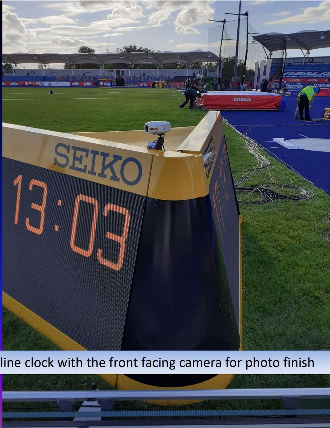
Finish line clock with the front facing camera for photo finish
